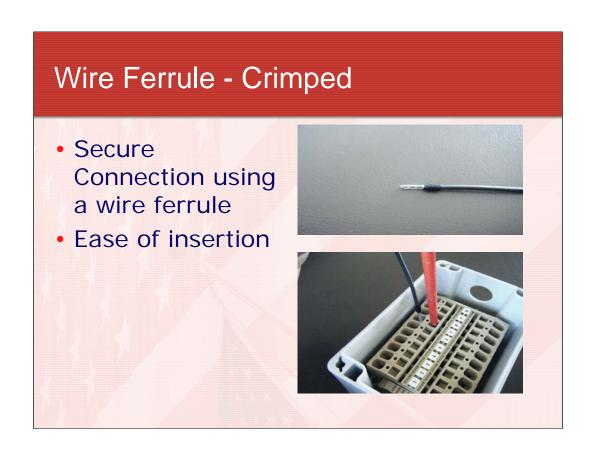
After crimping the Wire Ferrule onto the conductor, it is ready to be inserted into a device or a Terminal block. Inserting the conductor into a Terminal Block is now much easier and more secure when using a Wire Ferrule.
