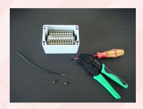
American Electrical offers all types of Insulated, Non-insulated, Twin wire and assortments for wire ferrules. Wire Ferrules are a Tin plated Copper tube (with or without an insulation sleeve) that are mechanically crimped to the end of a conductor to secure the strands. Crimping the wire ferrule to the conductor insures that stands do not splay, increases conductivity and reduces resistivity while improving the overall integrity of the connection.
