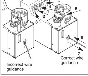
Figure 17 Crimp the wire
