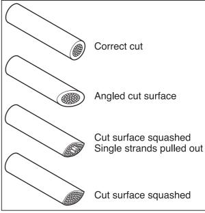
Figure 8 Cut wires to length
