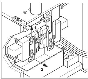
Figure 40 Remove the holding fixtures for the litz wire centring funnel
