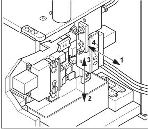
Figure 25 Changing the sleeve turning block
