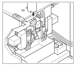
Figure 39 Remove the sleeve holder
