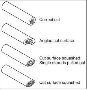
Figure 16 Cut the wire to size
