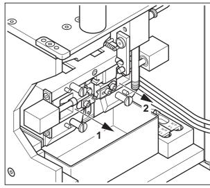
Figure 41 Remove the stripping blades
