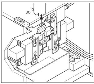
Figure 45 Remove the sleeve holder
