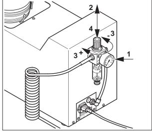
Figure 33 Check the air pressure
