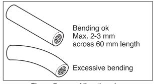
Figure 7 Align the wires
