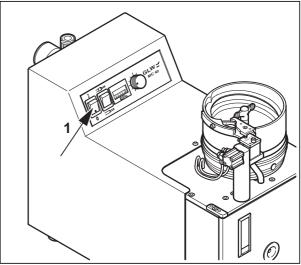
Figure 29 Check the mains lamp
