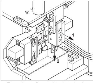
Figure 34 Remove the sleeve turning
