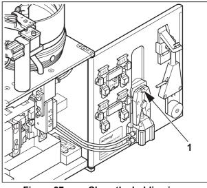
Figure 37 Clean the holding jaws
