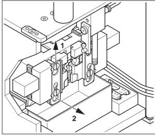
Figure 46 Remove the holders for the litz wire centring funnel
