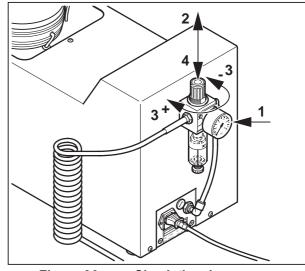
Figure 36 Check the air pressure
