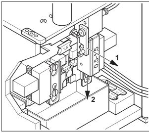
Figure 38 Remove the sleeve turning
