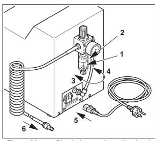
Figure 21 Check the condensation level
