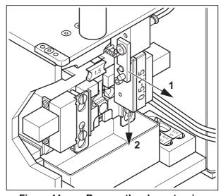
Figure 44 Remove the sleeve turning
