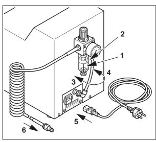
Figure 13 **Check condensation**
