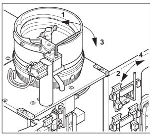
Figure 28 Changing the separator plate
