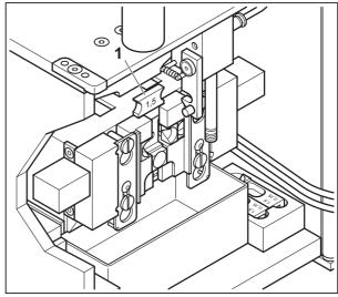
Figure 35 Check the sleeve holder
