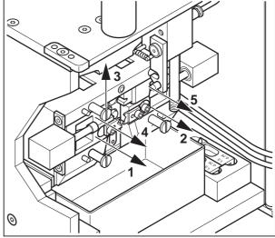
Figure 47 Remove the pressing jaws
