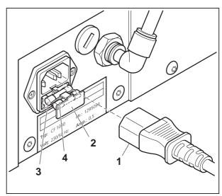
Figure 30 Check the mains fuse
