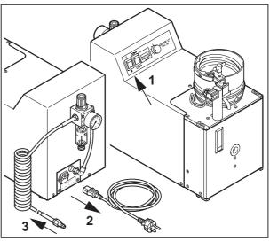
Figure 19 Switch off the MC 40
