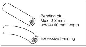
Figure 15 Align the wire
